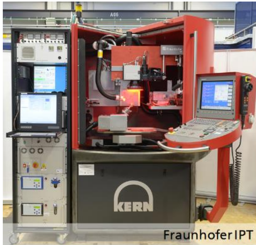
Figure 1 Existing 5-axes laser machine tool updated for laser-based lacquer ablation.
